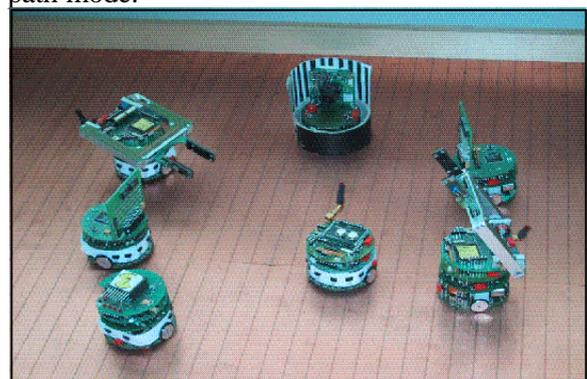
Figure 2. Seven Kheperas equipped with different devices.
