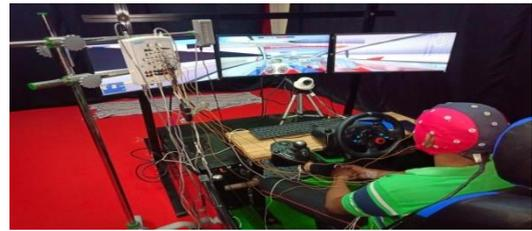
Figure 1. Driving simulator setup.
