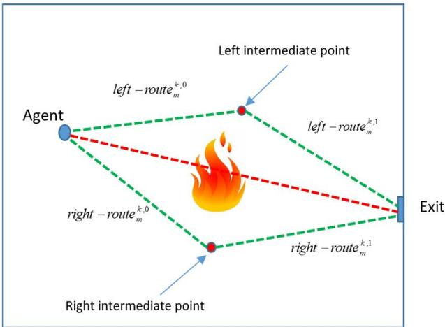
Figure 2. The agent's ability of detecting left and right intermediate points and composing left and right routes.
