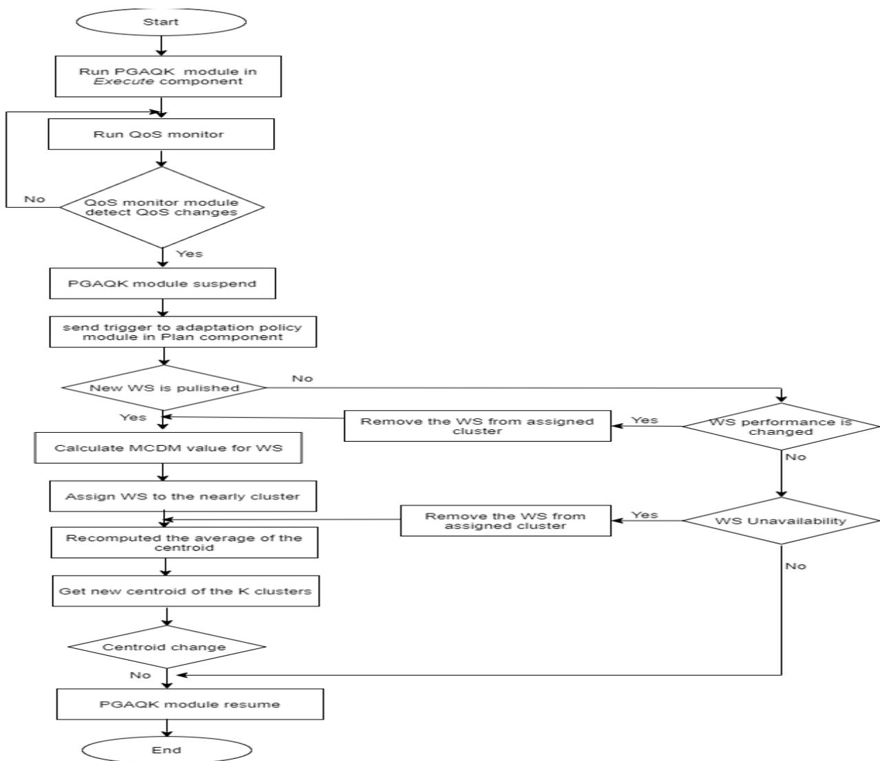
Figure 1. The flowchart of our proposed self-healing model.
