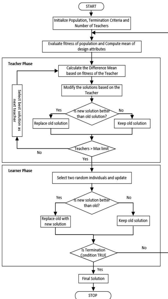
Figure 4. Workflow of the ITLBO algorithm.
