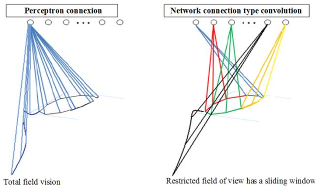
Figure 4. Connections' illustrations in MLP and TDNN.
