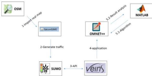
Figure 1. Guidelines for VANET simulation.
