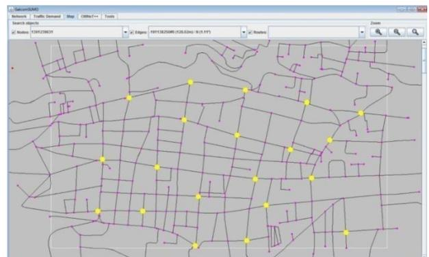
Figure 9. Each possible location for RSU appears as yellow circles on the map layout.
