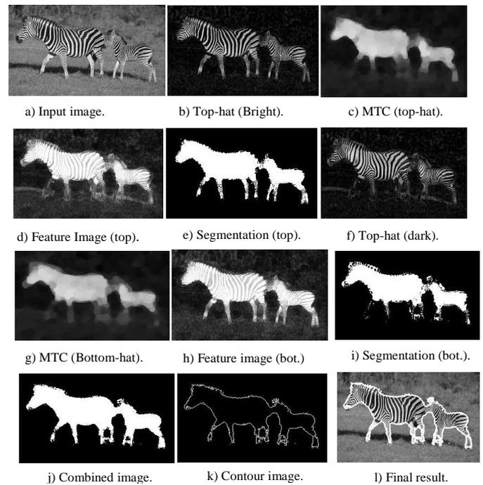
Figure 4. Intermediate images for segmentation of zebra image.
