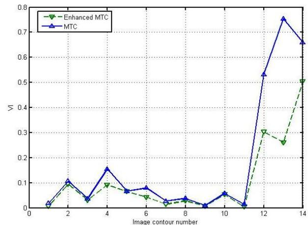
Figure 12. Variation Of Information (VOI) is low for enhanced MTC. When the shape complexity increases it reduces further thus boundary localization improves very much.
