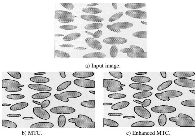
Figure 6. Boundaries are much more localized in enhanced MTC and much nearer to original 5-a.
