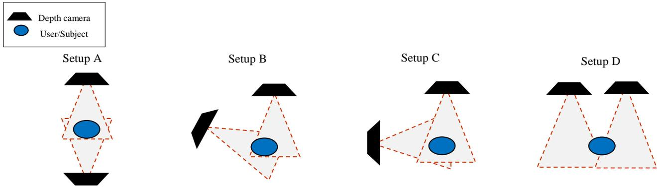
Figure 2. Multiple Kinect setup for experiments.
