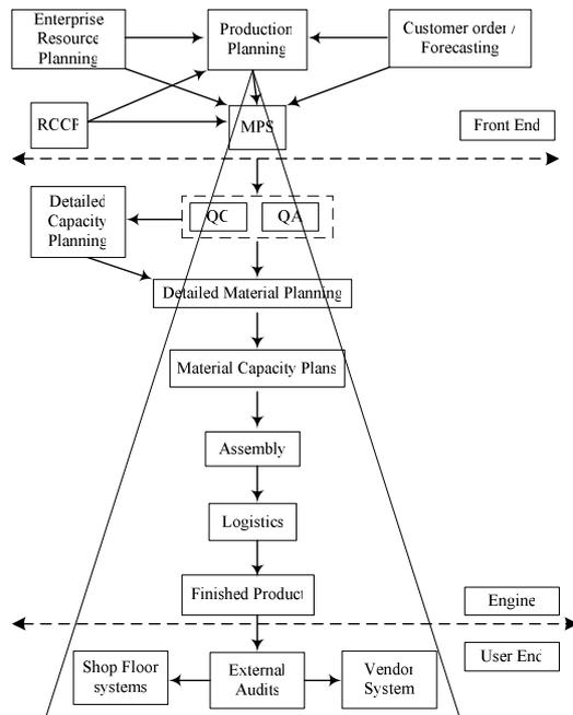
Figure 9. JIT pull logic for customer demand.
