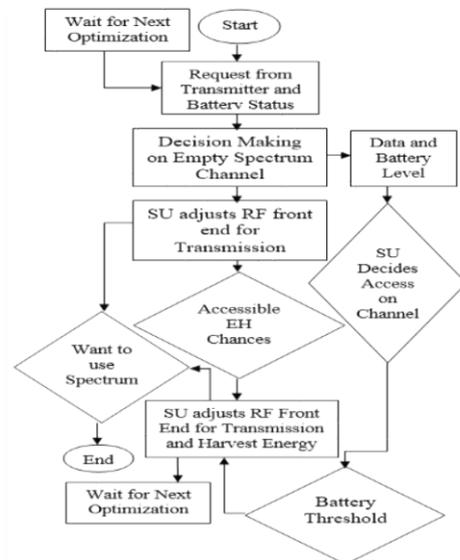
Figure 3. Flow chart of RF energy harvesting system.
