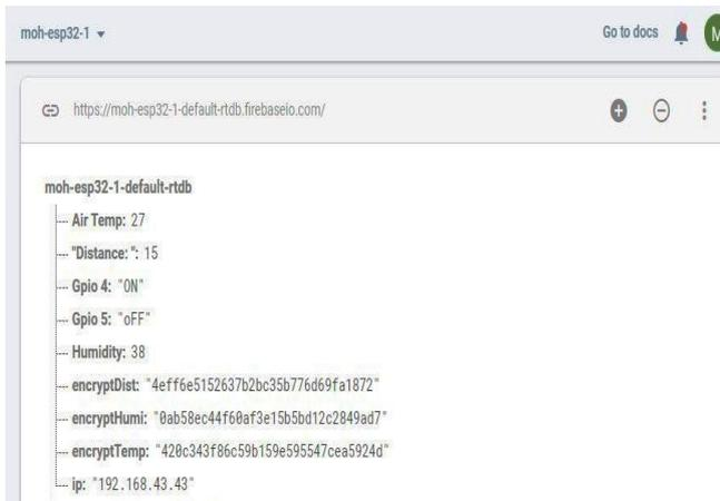
Figure 16. Data sensors on Firebase web page.
