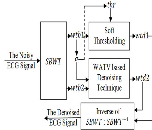
Figure 2. The flowchart of the proposed ECG denoising approach.
