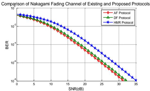
Figure 12. Comparison of nakagami fading channel with existing protocols and proposed HMR protocol.
