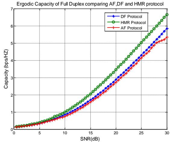
Figure 9. Ergodic Capacity of full duplex comparing AF, DF, and proposed HMR protocol.
