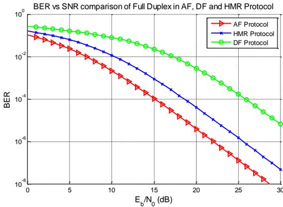
Figure 7. BER vs SNR comparison of full duplex in AF, DF, and proposed HMR protocol.
