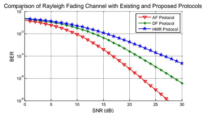
Figure 10. Comparison of rayleigh fading channel with existing protocols and proposed HMR protocol.
