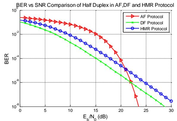
Figure 6. BER vs SNR Comparison of Half Duplex in AF, DF and proposed HMR Protocol.
