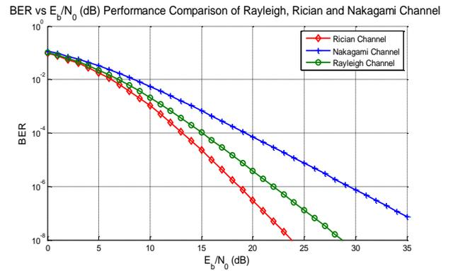
Figure 13. BER vs  $E_b/N_0$  performance comparison of rayleigh, rician and nakagami channel.
