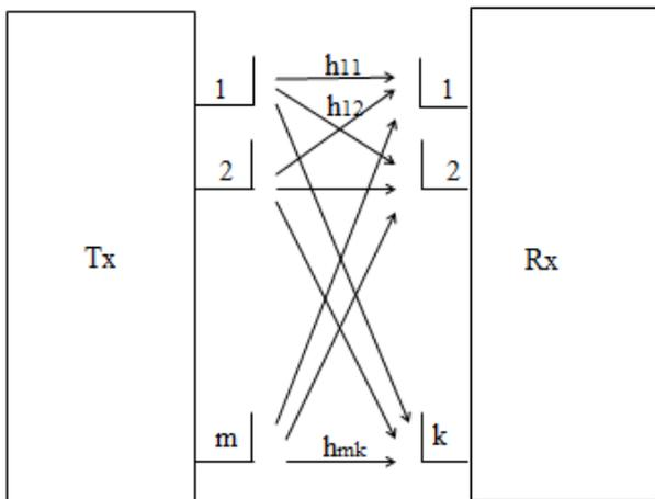
Figure 1. MIMO system model.
