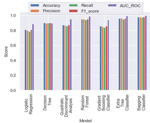
Figure 5. Comparison of machine learning techniques for predicting smart grid stability.
