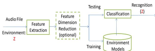
Figure 1. Block diagram of environment recognition from audio files.
