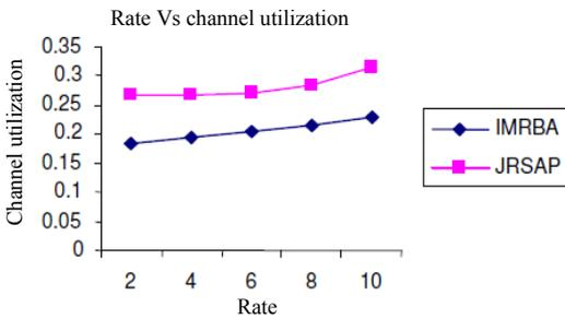
Figure 10. Rate Vs utilization.
