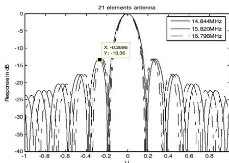
Figure 1. Plane wave response of a linear array with input frequency.
