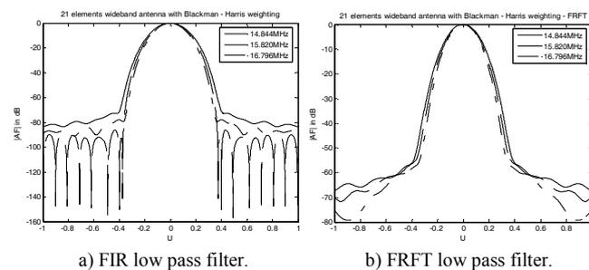
Figure 9. Response of 21-element wideband antenna array designed with Blackman-Harris weights.
