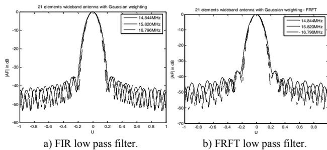
Figure 6. Response of 21-element wideband antenna array designed with Gaussian weights.
