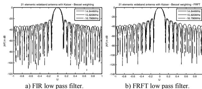
Figure 8. Response of 21-element wideband antenna array designed with Kaiser-Bessel weights.
