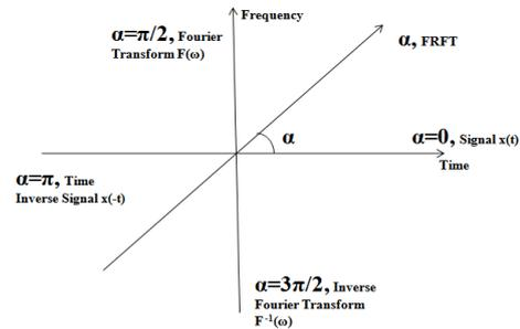
Figure 3. Rotation of signal in time frequency plane with an angle  $\alpha$ .
