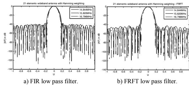
Figure 7. Response of 21-element wideband antenna array designed with Hamming weights and FRFT Low Pass Filter.
