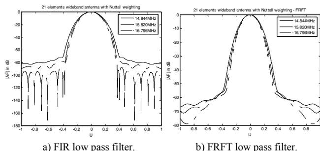
Figure 10. Response of 21-element wideband antenna array designed with Nuttall weights.
