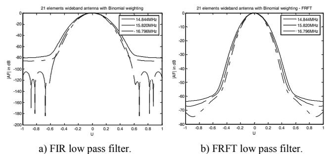
Figure 5. Response of 21-element wideband antenna array designed with binomial weights.
