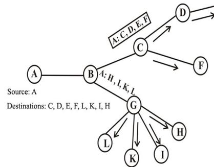
Figure 1. XCAST packets delivery mechanism.
