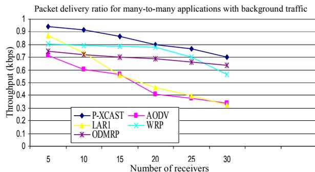
Figure 19. Packet delivery ratio for many-to-many applications with background traffic.
