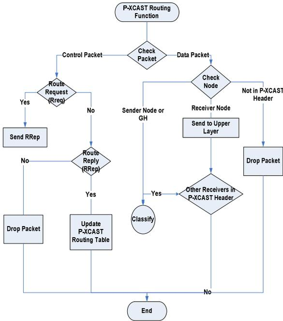
Figure 7. P-XCAST routing function.
