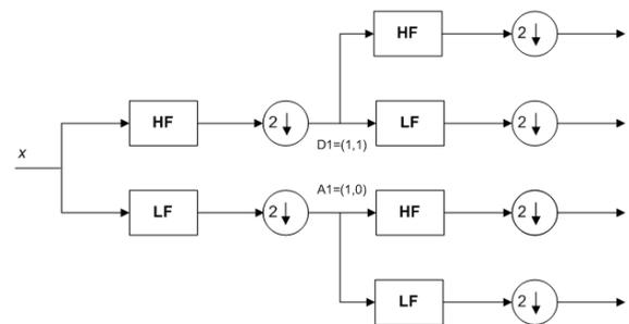
Figure 1. Wavelet packet decomposition of level two.
