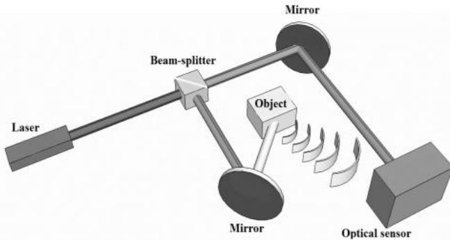
Figure 1. Laboratory setup for digital hologram recording process.
