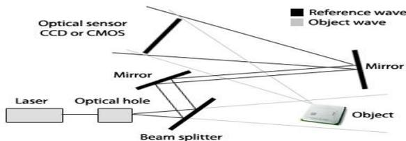
Figure 2. Laboratory setup for recording holograms with offset errors.
