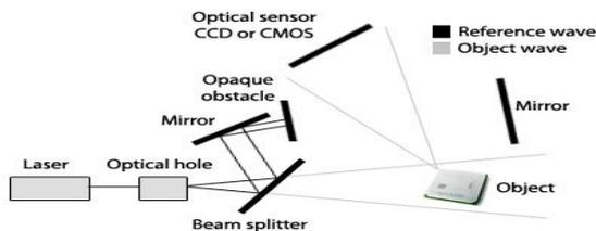
Figure 3. Laboratory setup for recording object wave.
