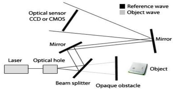
Figure 4. Laboratory setup for recording reference wave.
