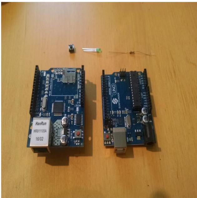
Figure 3. Arduino uno and ethernet controller.
