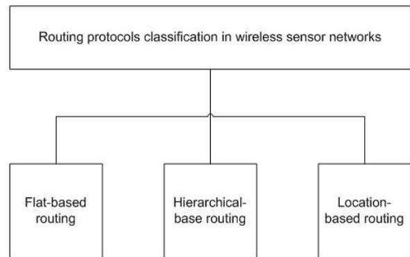
Figure 3. Routing protocols classification for WSN.
