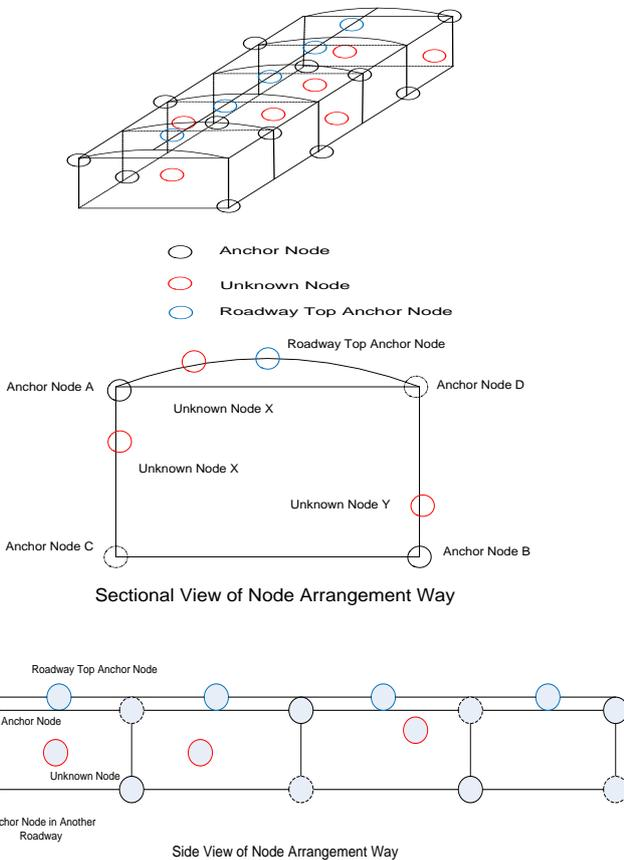
Figure 2. Arrangement rule, sectional view and side view of new anchor nodes.
