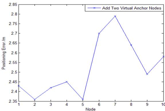
Figure 9. Positioning effect as virtual anchor nodes in the plane of roadway wall were considered.
