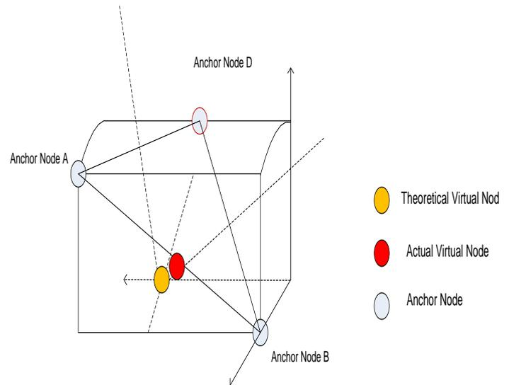
Figure 6. Establishment of virtual anchor nodes in the plane composed of any wall anchor node and top anchor nodes.
