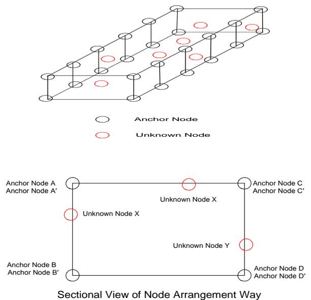
Figure 1. Arrangement rules and sectional view of anchor nodes in roadway.
