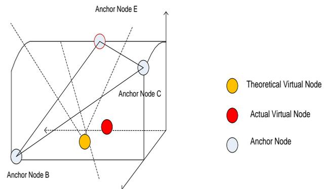
Figure 7. Establishment of virtual anchor nodes in the plane composed of neighboring area wall anchor nodes and top anchor nodes.
