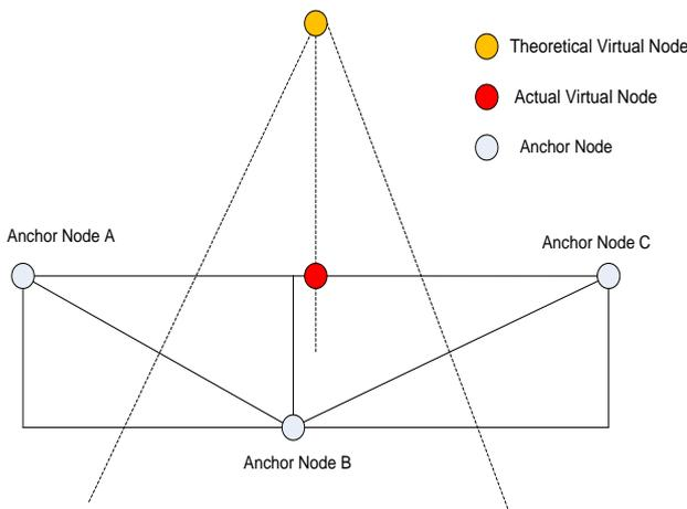
Figure 5. Establishment of virtual anchor nodes in the plane composed of roadway wall anchor nodes.
