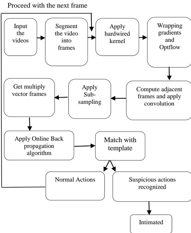
Figure 2. Work flow of the proposed model.
