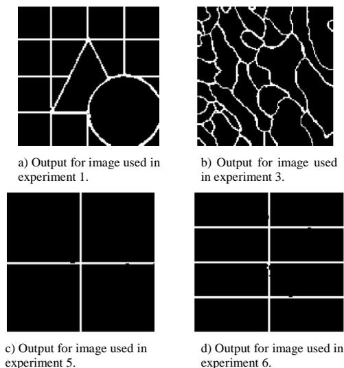
Figure 8. Edge detection output of the test images with noise variance 0.01.
