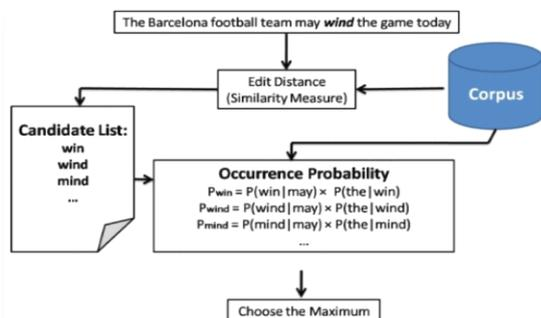
Figure 2. The schematic design of RWSC algorithm.
