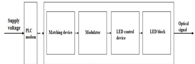
Figure 3. Block diagram of a transmitting module of VLC technology with a PLC interface.
