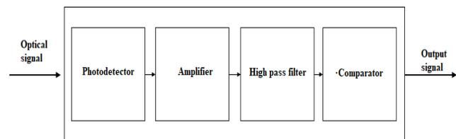
Figure 4. Block diagram of the receiving module of VLC technology with PLC interface.
