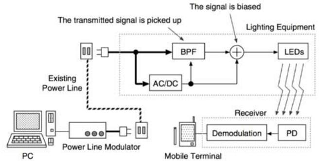
Figure 1. Visible light communication system.
