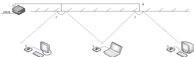
Figure 2. The principle of operation of VLC technology with a PLC interface (1-PLC adapter, 2-VLC transmitter module, 3-VLC receiver module, 4-power line).
