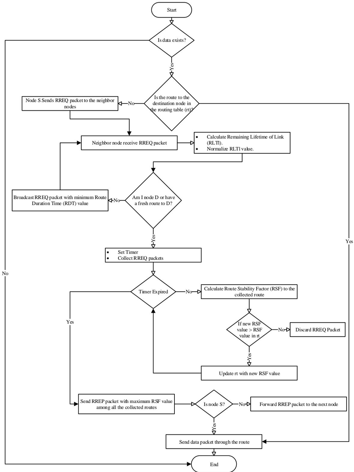
Figure 3. The routing process of the proposed scheme.
