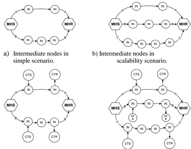
c) intermediate nodes and cross traffic in simple scenario. d) intermediate nodes and cross traffic in scalability scenario.
