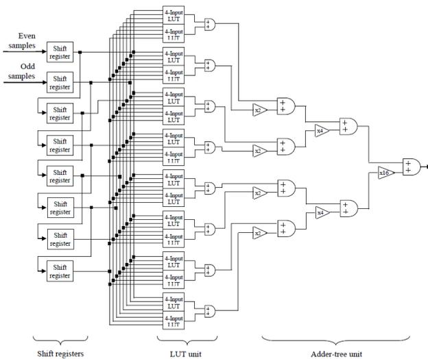
Figure 5. VLSI architecture of DA-based wavelet computation.
