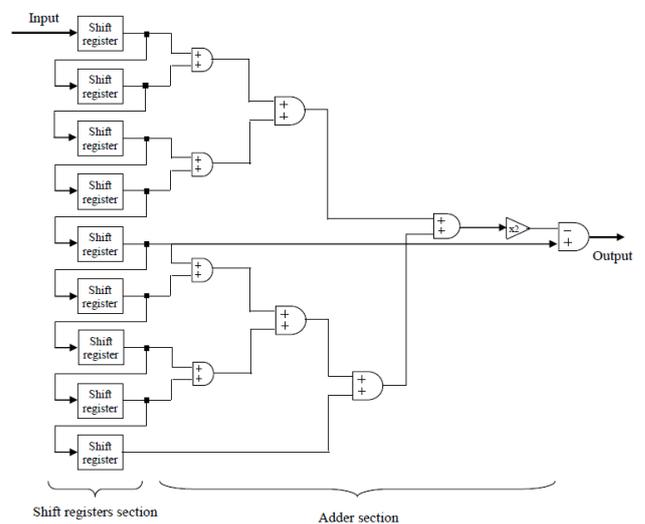
Figure 7. VLSI architecture of DPCM transformation.
