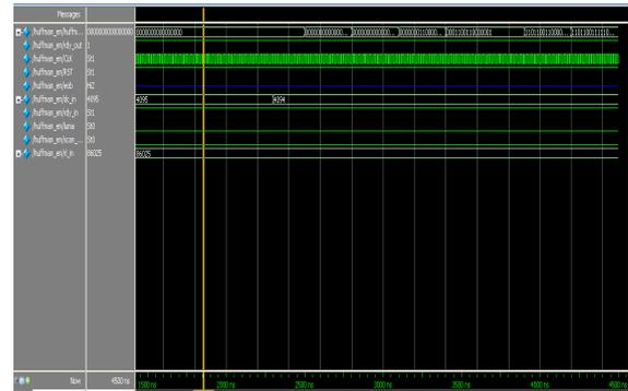
Figure 11. Functional verilog simulation of Huffman encoding.
