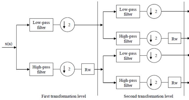
Figure 3. Wavelet computation with  $R_w$  block.
