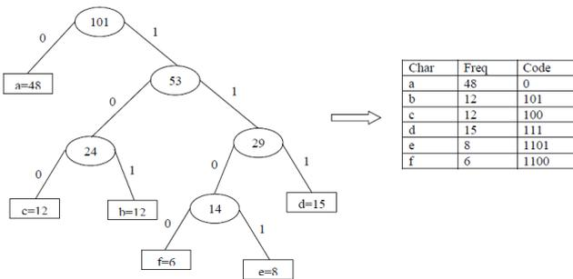
Figure 8. Huffman encoding procedure.
