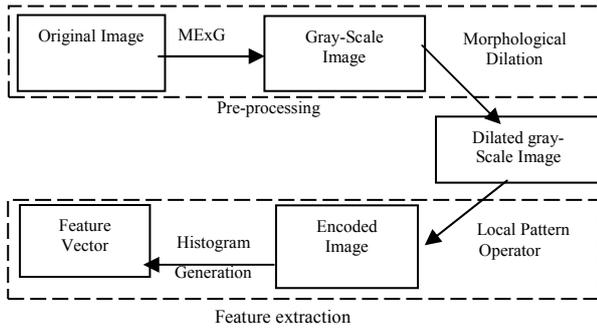
Figure 7. Illustration of feature vector generation process.
