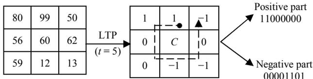
Figure 2. Illustration of the LTP encoding process (the LTPcode is 1100(-1)(-1)0(-1) and the corresponding positive and negative patterns are 11000000 and 00001101, respectively).
