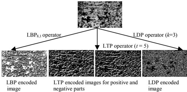
Figure 8. Encoded image representations obtained by applying different local pattern operators.
