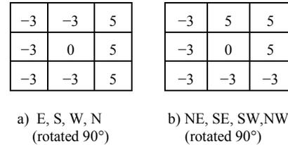
Figure 3. Kirsch eight directional edge response masks (different orientations are obtained by rotating these masks by  $90^\circ$ ).
