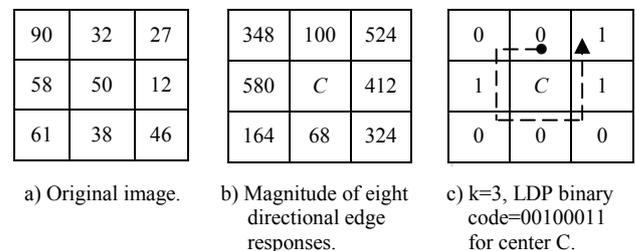
Figure 4. Illustration of the LDP encoding process.
