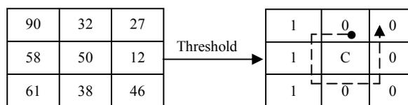
Figure 1. Illustration of the LBP encoding process (the LBP binary code for pixel C is 01110000).
