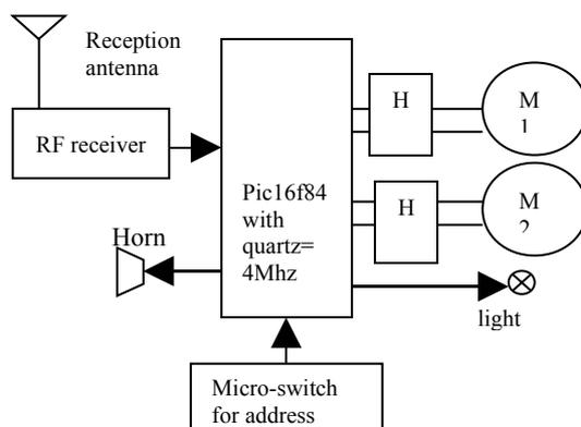
Figure 3. Autonomous robot block diagram.
