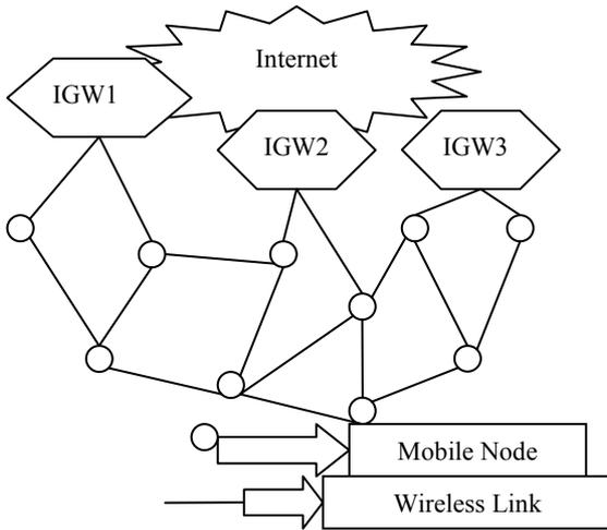
Figure 1. Mobile ad hoc network connectivity with Internet.
