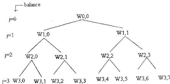
Figure 3. Wavelet packet binary tree.
