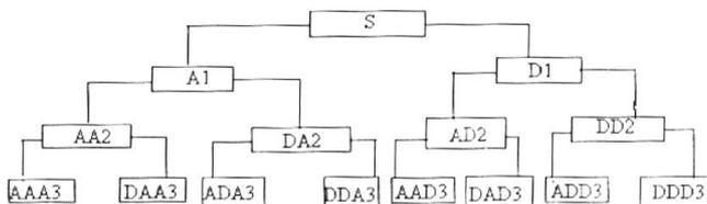
Figure 4. Detailed and approximation nodes.
