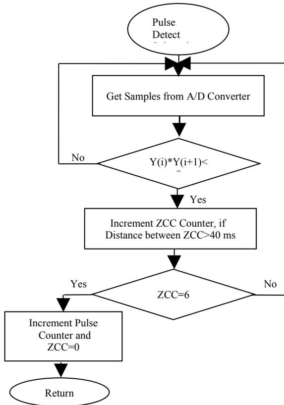
Figure 5. Flow chart of zero crossing algorithm.
