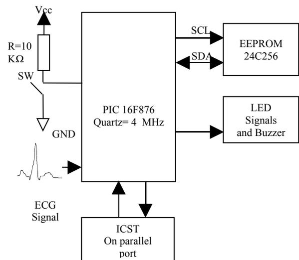
Figure 4. Configuration of the system.
