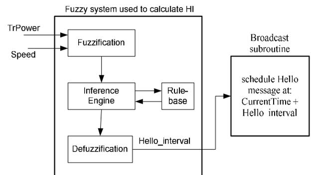
Figure 4. Block-diagram for the basic elements of the fuzzy system.
