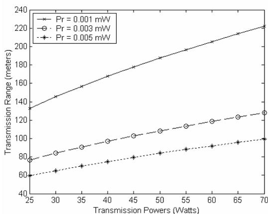
Figure 1. Transmission range versus transmission power.
