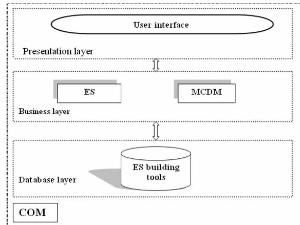
Figure 2. Three-tire architecture of the proposed system.
