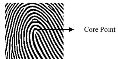
Figure 1. The reference point on the convex ridge.
