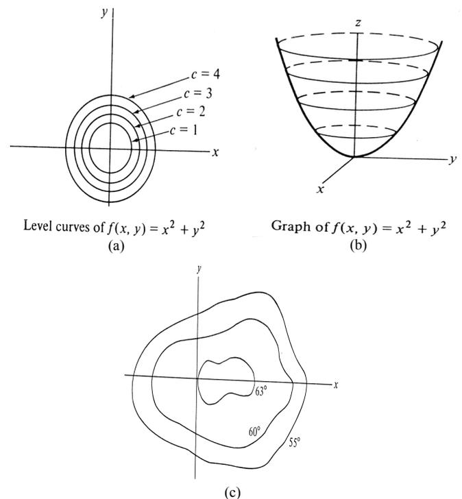
Figure 1. Isotherm and function  $f(x, y) = x^2 + y^2$  level curves.
