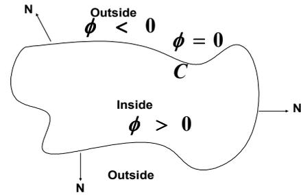
Figure 3. Curve  $C = \{(x, y) : \phi(x, y) = 0\}$  propagating in normal direction.
