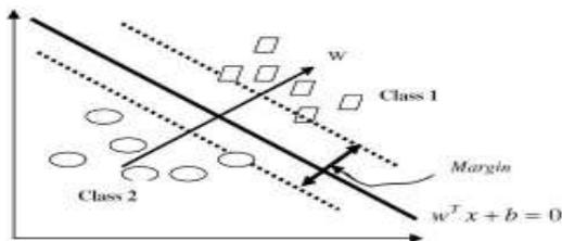
Figure 4. Hyperplane with the maximal margin by a linear SVM.
