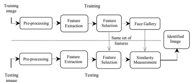
Figure 1. Basic block diagram of an FR system.
