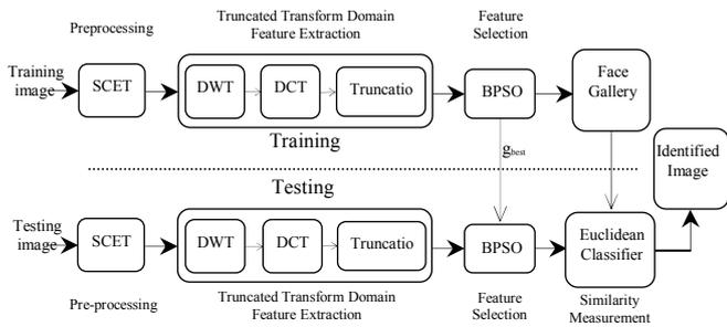
Figure 5. Block diagram of the proposed FR system
