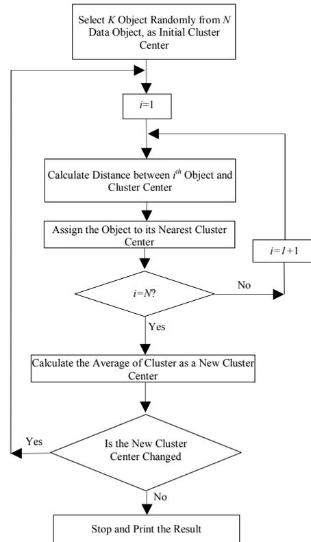
Figure 1. Flowchart of the K-means.
