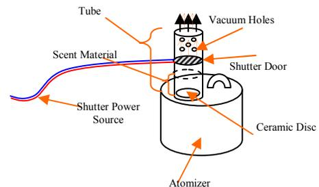
Figure 7. The atomizer with scent material and tube.
