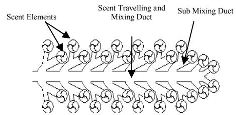
Figure 5. Arrangement of the scent element and duct pathway.
