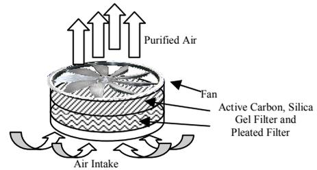
Figure 4. Purification and odor neutralizing filter.
