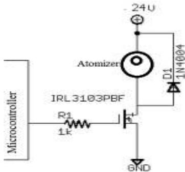
Figure 3. Typical scent element driving circuit.
