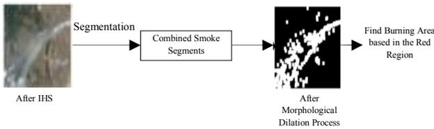
Figure 3. Discovering burning areas from the smoke segments using directional analysis.
