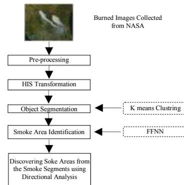
Figure 1. Overall block diagram of burning area identification technique.
