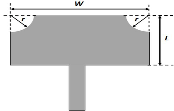
Figure 2. Rectangular microstrip antenna with quarter circular slots.
