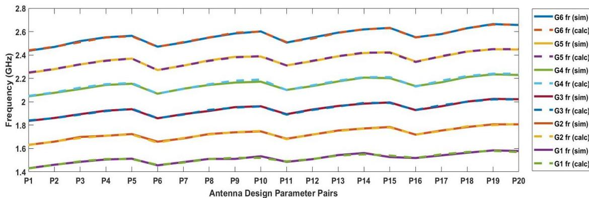
Figure 3. The comparison of simulated (solid) and calculated (dashed) frequencies for each group (Group 1 (bottom) to Group 6 (top)).
