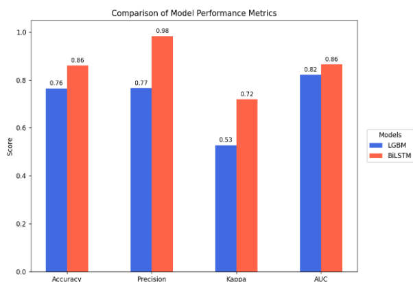
Figure 22 LGBM vs. BiLSTM comparison based on accuracy, precision, kappa, and AUC score.
