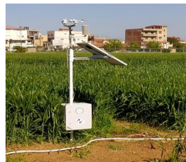
a) Sensor's station (Arduino+LoRa SX1278+sensors).
