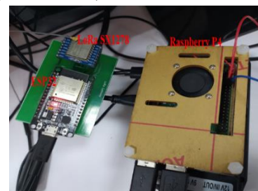
b) Gateway (RaspberryP4+ESP32+ LoRa SX1278).
