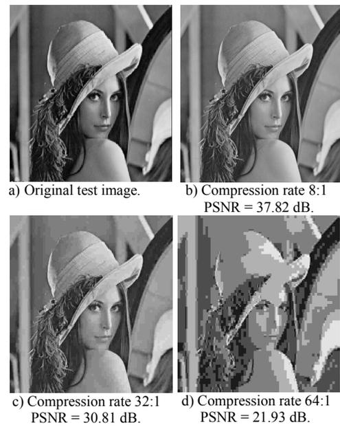
Figure 16. Simulation results using standard JPEG.
