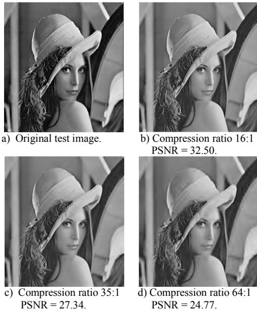
Figure 12. Simulation results using wavelet transform.
