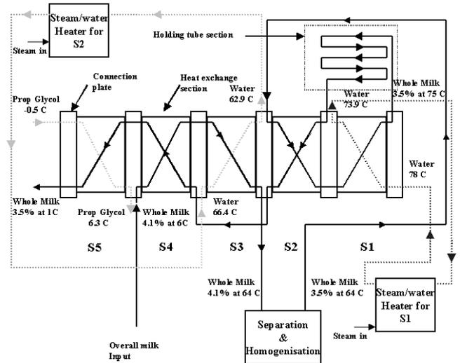
Figure 1. General layout of the pasteuriser plant.
